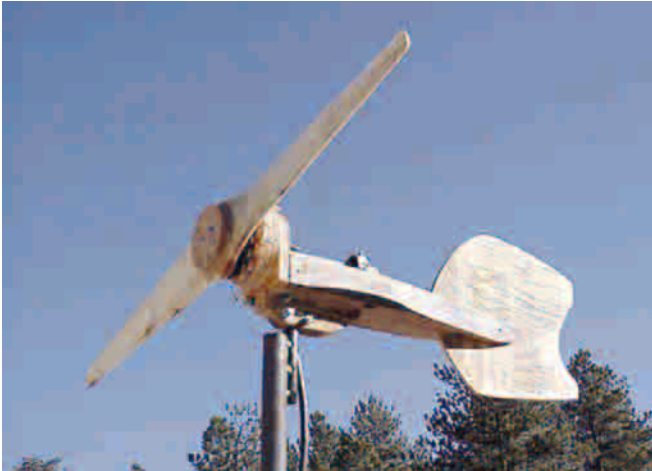
The next generation—the WoodAx is for permanent installation, and produces upwards of 300 watts in 30 mph winds.
