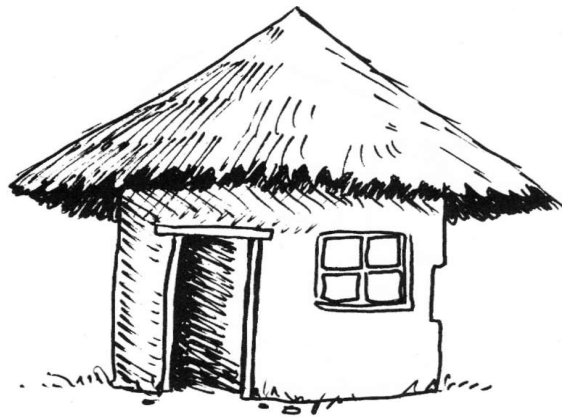
A thatched cone-shaped roof is very common on many African cob homes.
