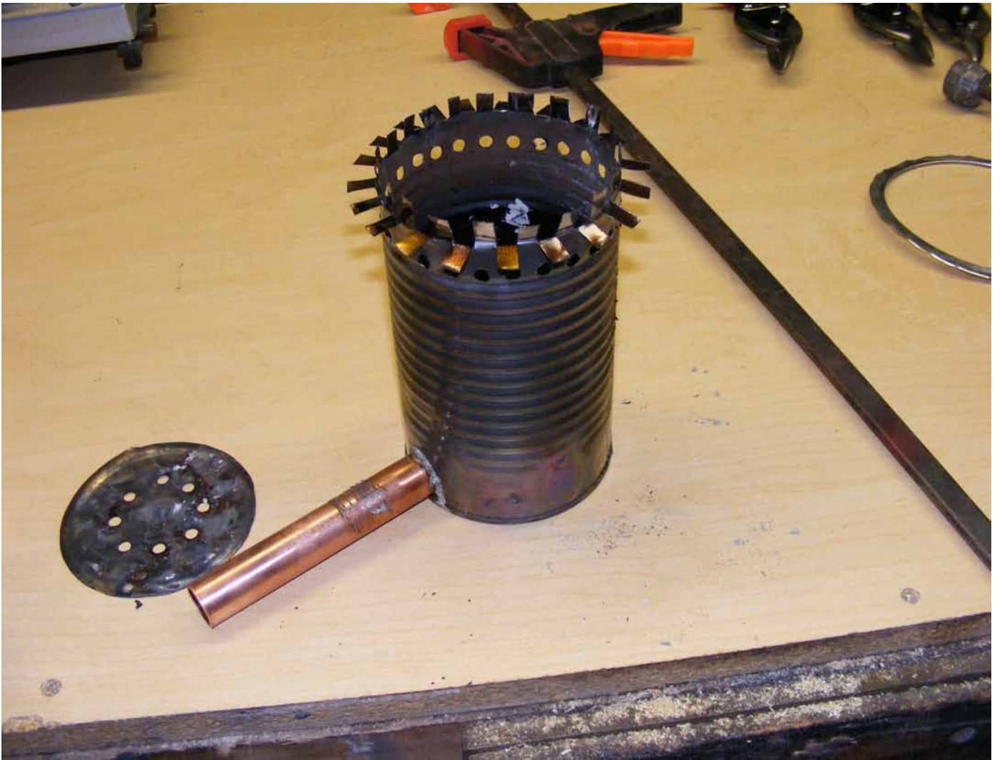
This is a picture of the burner after the concrete set up. The pipe will go through the secondary air can and the outside 5 gallon bucket.
