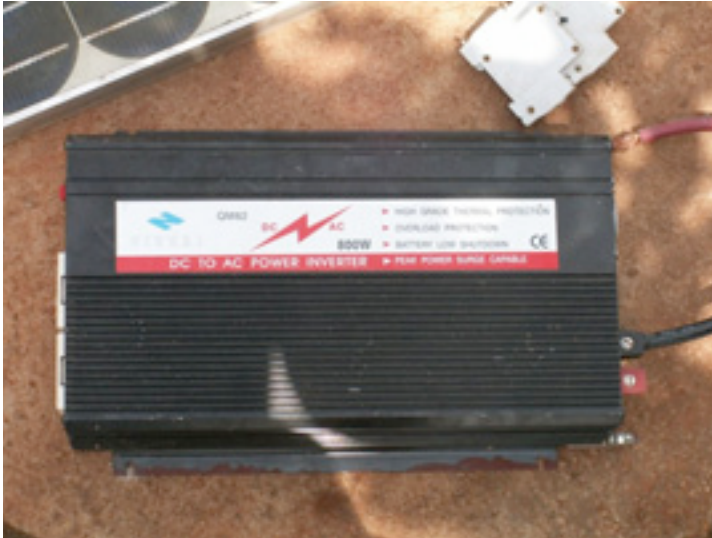
Figure 7.4: An 800 Watt DC/AC converter (power inverter)
