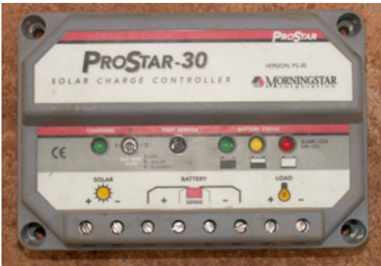
Figure 7.3: A 30 Amp solar charge controller
