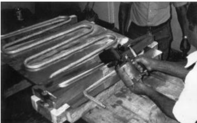
3: Take the burning soldering lamp and move it slowly to and for alongside the triangle.
