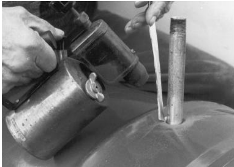
Photo 6: Then solder the piece of pipe in upright position securely into the hole.
