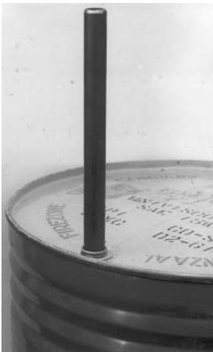
Fit the \frac{3}{4} " piece into the bungle. This is the vent.
