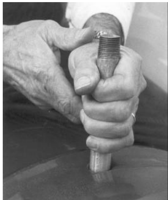
Photo 4: The thread-end of the pipe must be kept outside of the drum. All pipes stand perpendicular of the drum.
