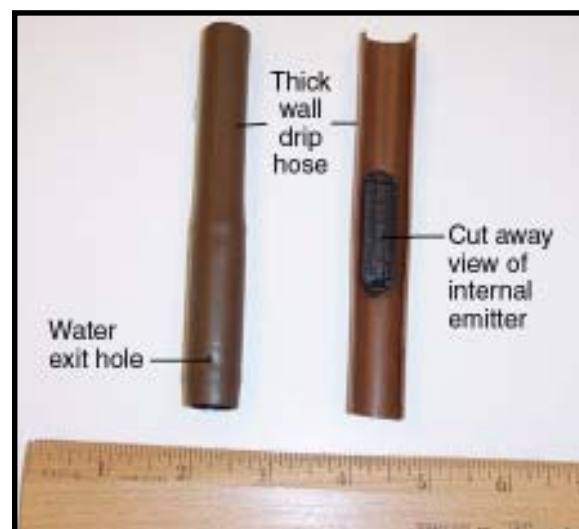
Figure 2. Thick wall drip hose specimen showing the water exit hole and the cutaway view of the internal emitter.
