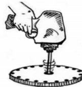
Drilling the holes in the centralizer
