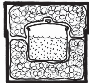
Figure 6 - Food Continues to Cook Inside the Insulated Haybox
