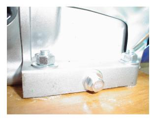
Now bolt the engine to the board, with the bolt heads and a flat washer on the bottom of the board, and flat washer, lock washer, and nut on the engine legs. We used round head bolts, but next time I'd use hex head to keep the bolts from turning when tightening.
