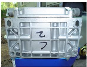
Take a sheet of paper and place it on the bottom of the engine. Poke a pencil through the mountings holes on the bottom of the engine to create your mounting hole template. Then place the paper on the board, and drill the mounting holes.
