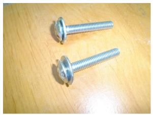
We used 4 bolts for the legs, with 2 flat washers, one lock washer, and nut for each of the leg bolts. Another 4 bolts, with lock washers for bolting the alternator bracket to the crankshaft face, and two bolts for the alternator, one with 2 flat washers, a lock washer and a nut, the other with a flat washer and a lock washer (the case is threaded, no nut).
