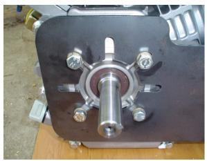
Next, we take the alternator bracket, and bolt it to the engine, using 4 bolts with lock washers. Then slide the pulley onto the shaft, with the key inserted, and slightly tighten the Allen screw. The pulley will be adjusted once the alternator is installed.
