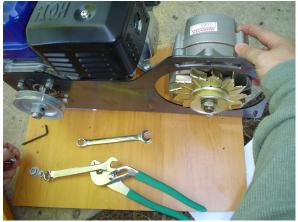
Now bolt in the alternator with the two alternator bolts. Install the belt, and adjust the tension, and tighten down the alternator.
