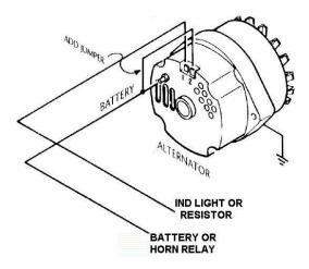
Depending on your alternator, you may have to install a 10 ohm 10 watt resistor between the number 1 terminal on the alternator and an ignition source to properly excite the alternator.
