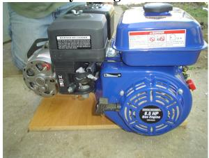
Our goal for this project is to build a engine driven battery charger for the off-grid home. A off-grid home is built around a battery bank, with a variety of ways to charge them. We use a combination of solar panels, wind turbines, and engine driven battery charger, the focus of this project. The battery bank then feeds a Inverter that provides "normal" 120vac house current. See the List of Materials in Appendix 4.
