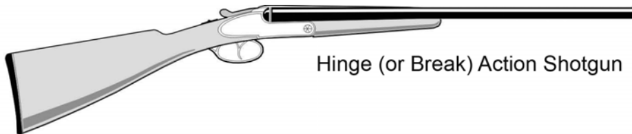
Figure 10. Types of firearms actions
